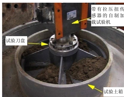
图 7 盾构刀盘掘进试验设备 Fig.7 Test equipment for cutterhead excavation
